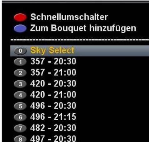
When pressing the **OPT (option)** in TV Mode, you see a list of Sub channels. Move the ▼ ▲ keys to the desired Sub channel and confirm with OK.
